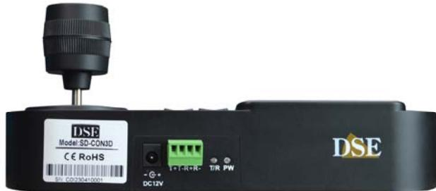
The R + R- terminals are available to connect another control unit such as a second console or a DVR.
